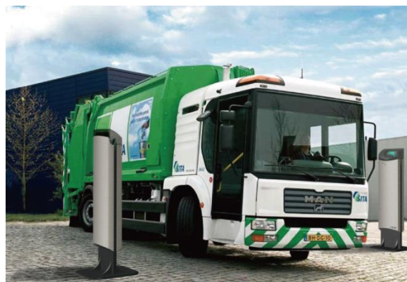
Waste truck radiation monitoring
